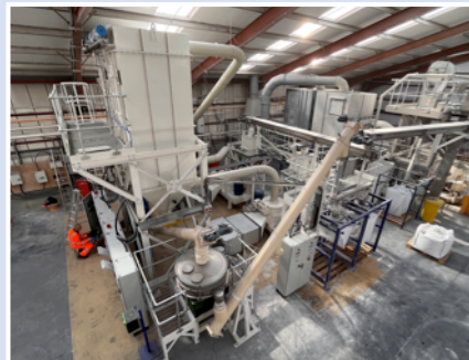
Twin ACM75 air classifier mill systems supplied by PPDS to a customer processing calcified seaweed
