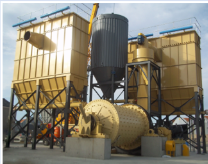
Drying, ball milling & classifying system for the processing of cement additives
