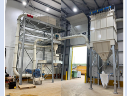
Milling and secondary classification system for protein shifting in legume flours
