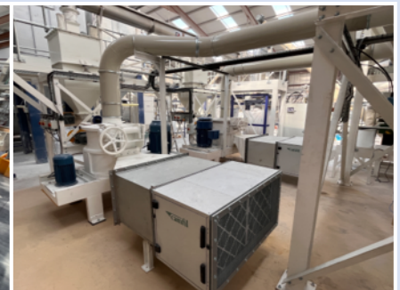
Twin ACM75 air classifier mill systems supplied by PPDS to a customer processing calcified seaweed
