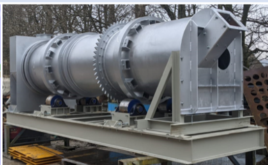
Rotary dryer designed and fabricated by PPDS as part of a system for processing glass cullet with a self-optimising remotely operated control system
