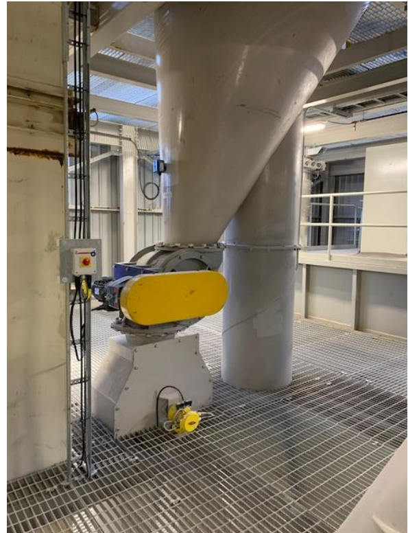
Classifier Rejects off-set cone with positional diverter valve allowing for regrind or transport via elevator to grits plant
