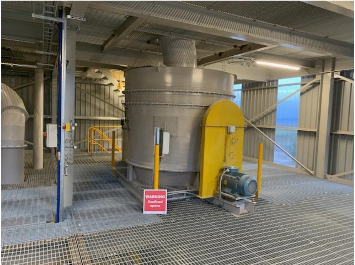
Whizzer Classifier for production of powders in the range of 99% passing 250 to 38 \mu m
