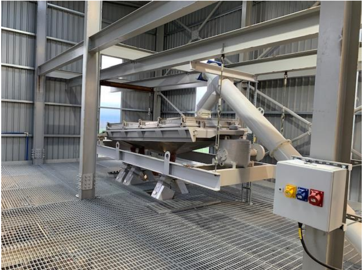
Rotex Locker Screen- precision screening of Mogensen undersized material
