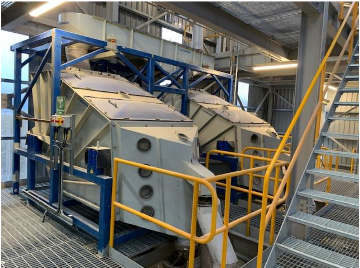
Mogensen Screens – screening grits between 4 and 1 mm
